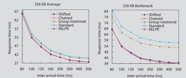
When operating in degraded mode, shifted declustering outperforms all other layouts in terms of both overall performance and bottleneck performance (performance of the slowest disk). This is illustrated in the two result graphs shown below:
